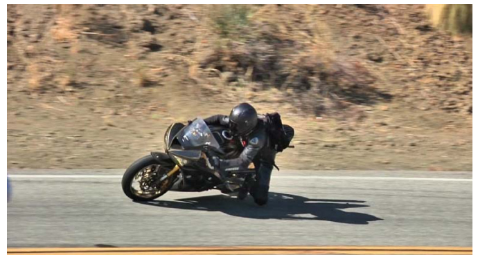
Figure 10. Contact with the Roadway Pulls the Rider's Left Knee Back and Pulls His Foot Off the Foot Peg
