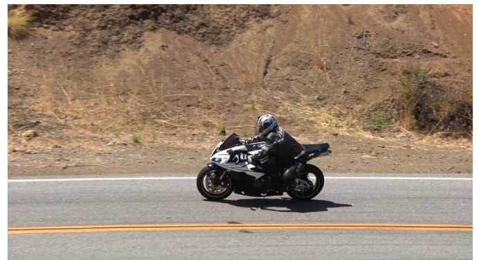
Figure 20. The Counterclockwise Yaw Ceases, the Motorcycle Yaws Clockwise and Rights Itself
