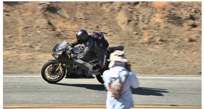
Figure 11. The Counterclockwise Yaw Ceases, the Motorcycle Yaws Clockwise and Rights Itself
