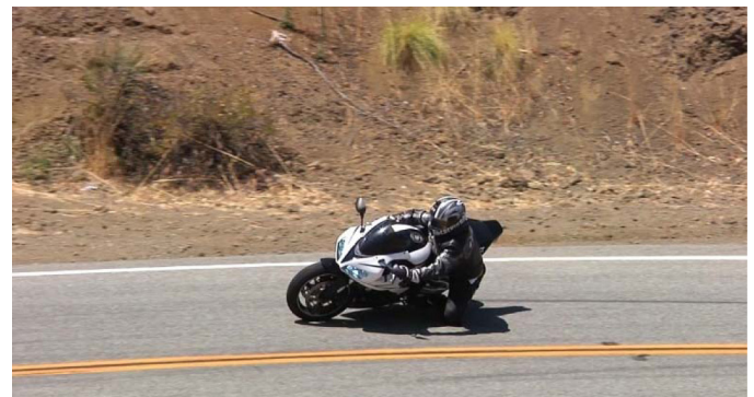
Figure 19. Right Side Leading Sideslip, Counter-Steer, and Tire Mark
