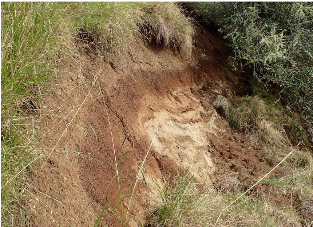
Fig. 11. Slip 7, on the western slopes, has exposed the freshest bedded Three Kings tuff (lower right) overlain by red-brown soil and then lighter brown terrace fill.
