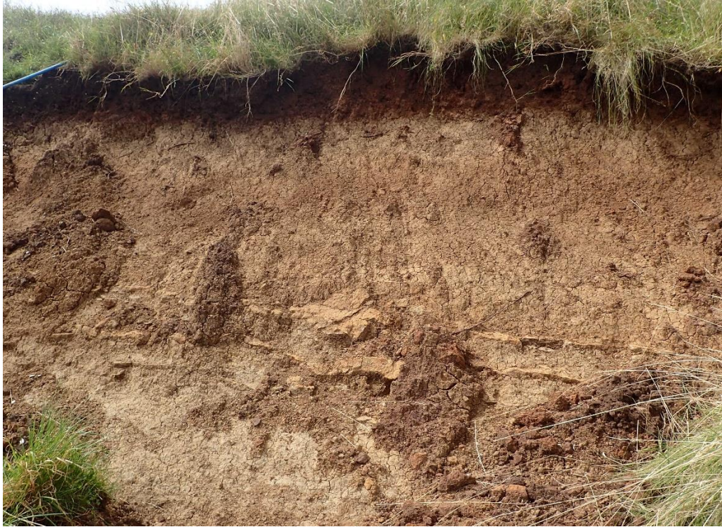
Fig. 10. Stratigraphy exposed in slip 2 with obvious beds of harder coarse tuff within finer tuff (all erupted from Three Kings Volcano) in the lower part of the scarp. This is overlain by a darker red-brown soil and at the top the lighter terrace fill.
