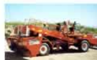
1988 The SupperChipper is the first production model chip spreader to offer true one-man operation, 30-inch-wide, deeply roughed aggregate belts, full computer control, and hydrostatic positive front-wheel drive.
