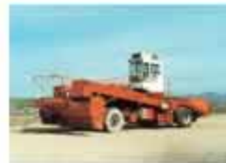
1985 BearCat introduces a self-propelled front-wheel-drive chip spreader with extendable distribution hopper. (Land-Speed Record for Self Propelled Chip Spreader - 66 mph)
