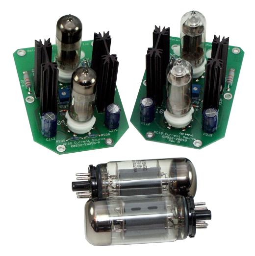
In its standard configuration the VK-33SE current sources use the Russian 6C19 tubes. That tube is basically a miniature version of the famous 6C33 tube, and provides, in our view, the best combination of sonic characteristics and electrical performance.
