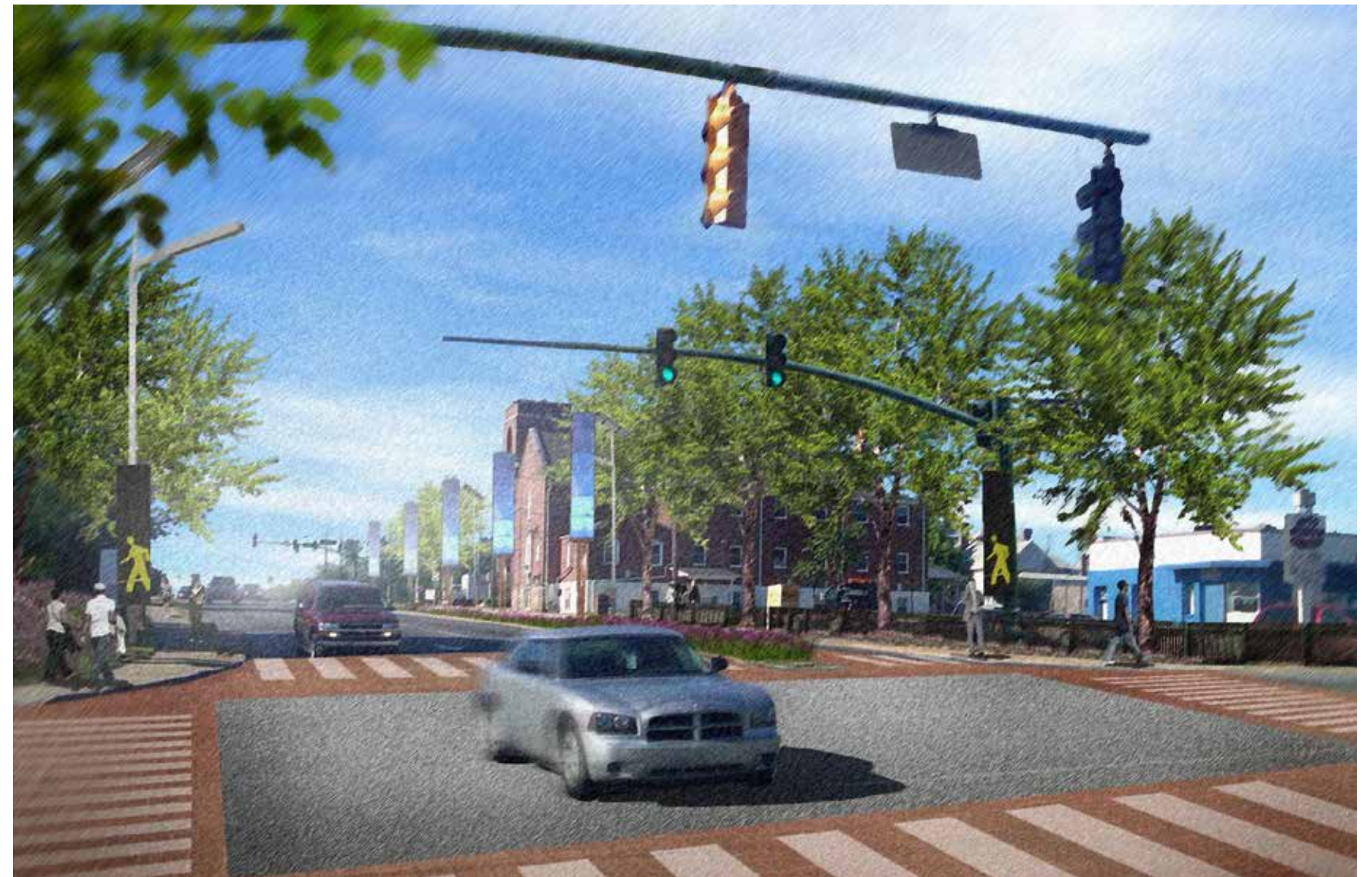
Example of Major and Minor Threshold intersection with special paving in crosswalk area, decorative light poles and signal poles, pedestrian art, and enhanced landscaping.
