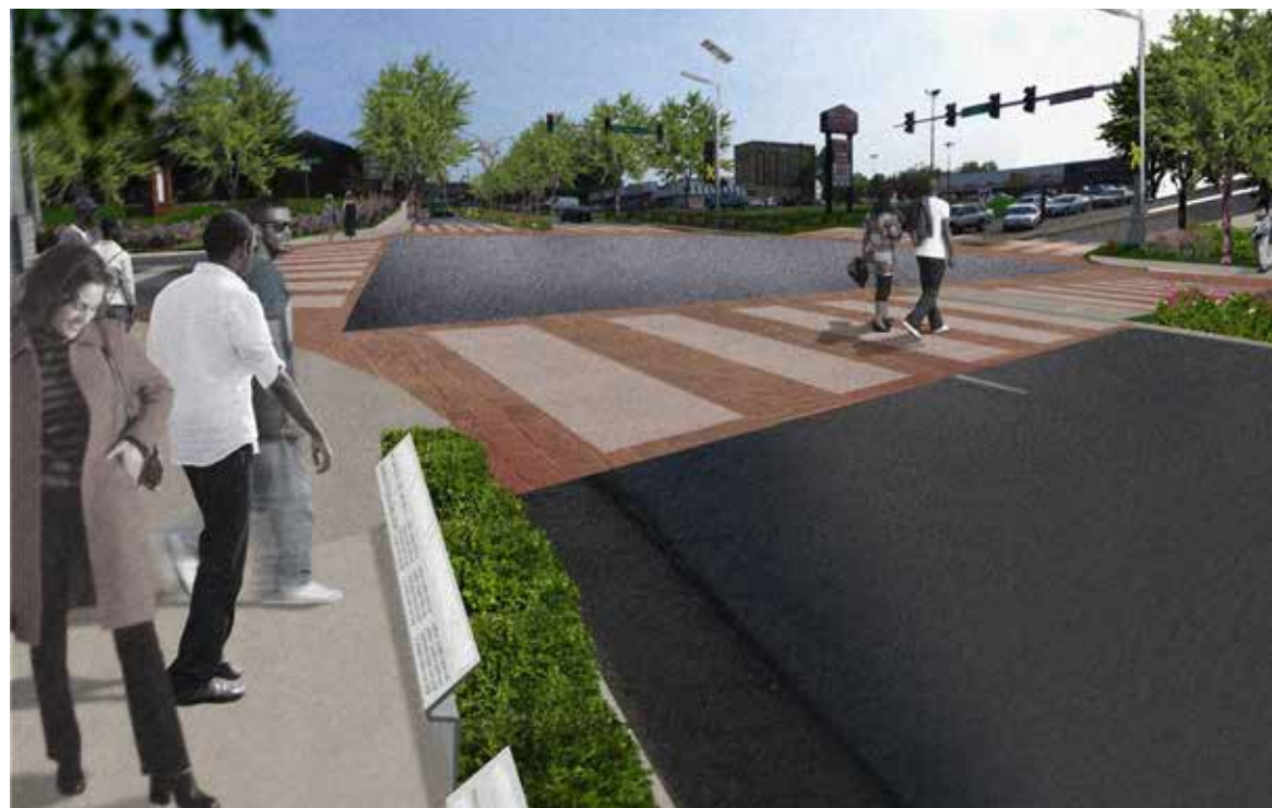
Example of Neighborhood Linkage zone intersection with special paving in crosswalk area, story-telling art next to sidewalk and enhanced landscaping. The story-telling art narrates important events, people or history and also provides a buffer from the busy street.
