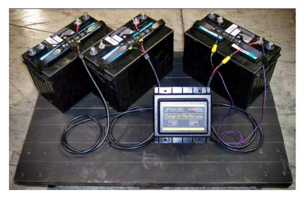
Locate the purple wire at the end of the starting battery cable assembly(this is not used on a CRS1). Using the supplied quick connector, attach the purple wire to any 12 volt source on the boat that is disabled when the boat is not in use. The purpose for this connection is to disable the **CRS** circuitry during times that the battery may be charged by other means (i.e., AC powered battery charger).
