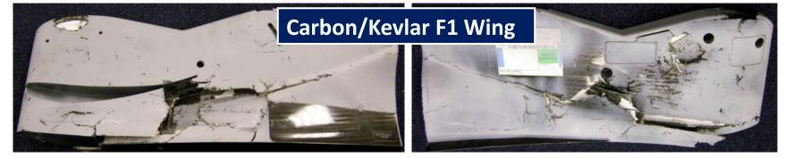
"falling weight impact tests and the mallet tests both showed the Innegra material to be equal to and generally superior to the Kevlar equivalent. This was manifested both in terms of resistance to damage and minimizing the size and quantity of debris".
