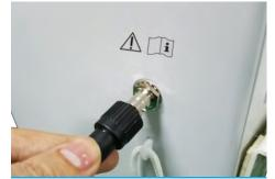
Figure 2. Connecting Coaxial Cable to the Cart
