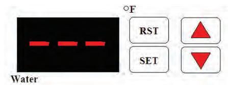
Figure 7. Shorted Temperature Sensor
