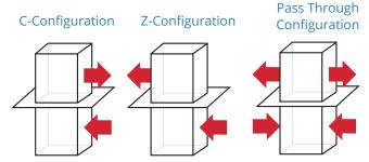
The Lift Configuration refers to the unloading and loading pattern of the lift. This lift allows for loading and unloading on the same side ("C"), from front to rear ("Z") or pass through.
