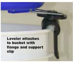
Once the Bowl is level, adjust the water flow so that the water is running at the top of the outer rim of the Bowl, but not overflowing. An even swirl pattern around centre cone is desired. Keep the water inside the Bowl; this will allow the vortex to maintain its strength and remove the black sands from your Bowl.
