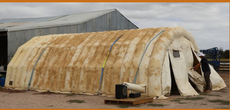
Polytunnel setup for sheep methane emissions measurement.
