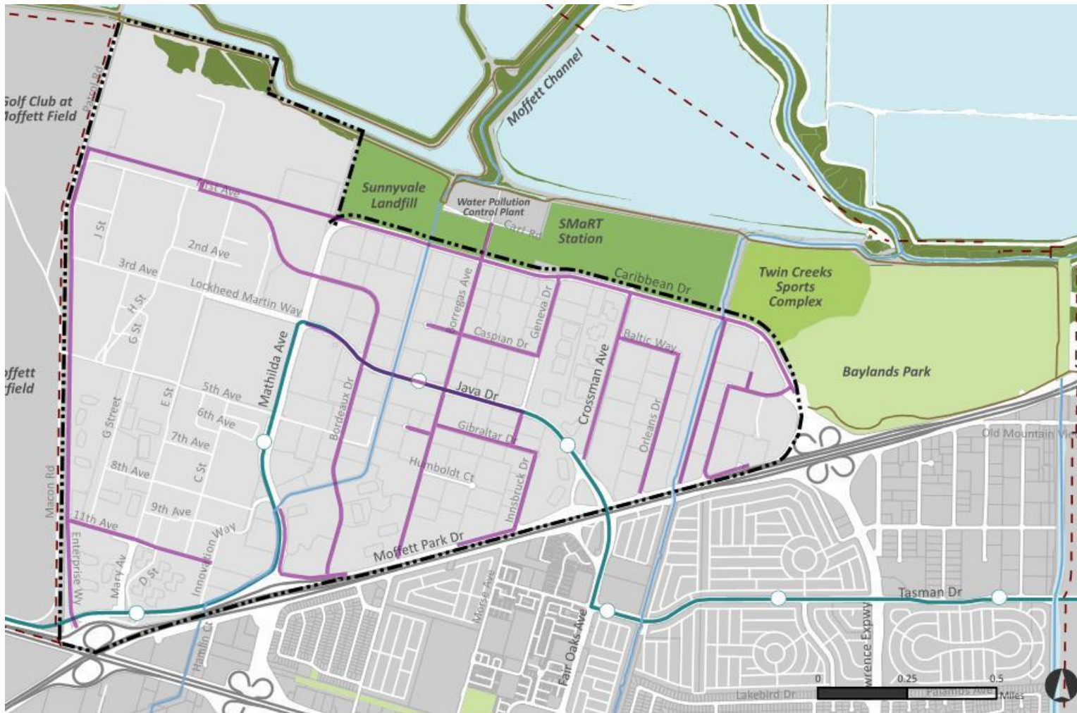
Figure 37. Recycled Water System
