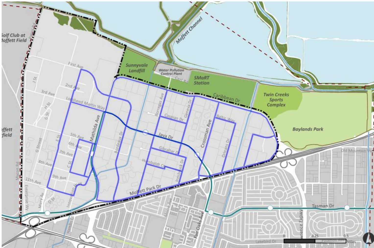
Figure 34. Water Distribution System
