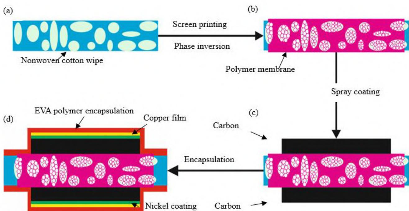
**Fig. 1:** Fabrication process of textile supercapacitor.
