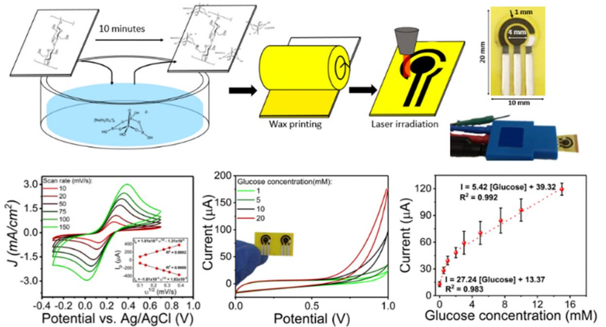
Fig.2. LIG on paper applied to electrochemical sensor production.
