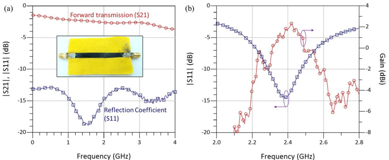
Figure 3. Biodegradable e-textile antennas and RF lines towards "green" chipless RF LAE: (a) A PEDOT:PSS printed transmission line for material characterisation and its measured transmission properties of the PEDOT:PSS line on a textile substrate; (b) The measured reflection coefficient and gain of a 2.4 GHz textile patch antenna using an all-polymer biodegradable radiating element.
