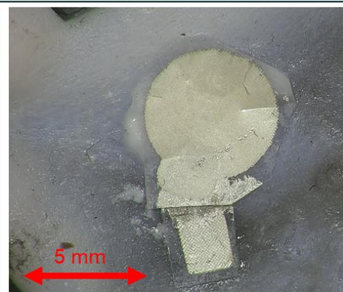
**Figure 2.** Electrical Characterisation and Modelling of Printed Electrodes on Mouse Skin
