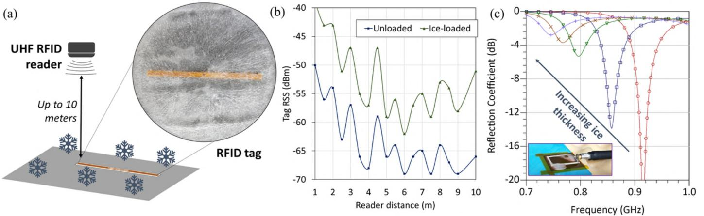
Figure 1. Robust large-area RF-enabled sensors for ice detection and monitoring in smart cities applications [1]: (a) illustration of the battery-free sensing system and a photograph of the ice-loaded RFID tag; (b) the measured sensor's performance showing at least 10 dB sensitivity; (c) the underlying operation principle where the ice "superstrate" shifts the resonant frequency; inset shows the dipole ice sensing antenna.
