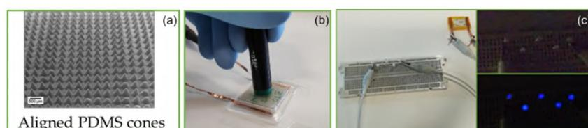
**Figure 1.** (a) SEM image of a micro-structured nanostructures@PDMS film. (b) Photograph of a nanogenerator. (c) Nanogenerator directly lighting up 5 LEDs by applying manual force.
