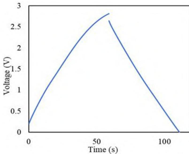
**Fig. 3:** Galvanostatic cycling tests ( $1 \text{ mA}\cdot\text{cm}^{-2}$ )
