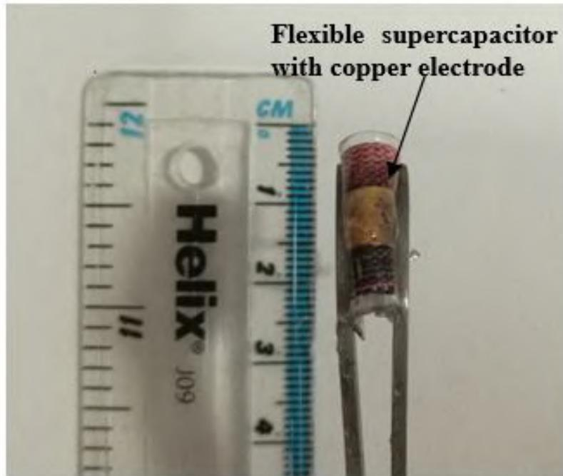
**Fig. 2:** Flexible supercapacitor under 180 degrees of bending conditions
