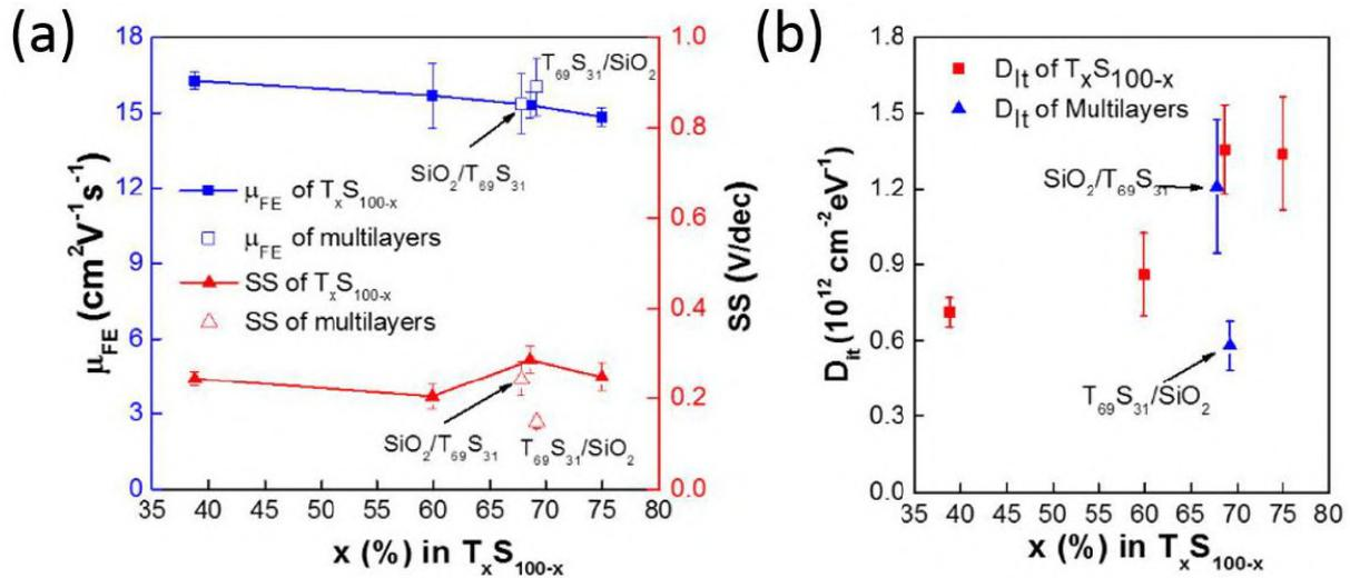
Figure 1 - (a) Field effect mobility and subthreshold slope and (b) trap density at the interface for TFTs employing the multicomponent and the multilayered dielectrics. Abbreviations: "T":  $T_2O_5$ , "S":  $SiO_2$ .
