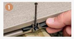
**PLACE CLIP IN GROOVE** Pinch the wings of clip together and slide the clip into the groove. The wings of the clip will expand, holding the clip in place until you're ready to fasten.
