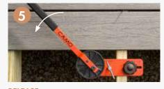
**RELEASE** Release pressure by moving the handle away from the deck board.
