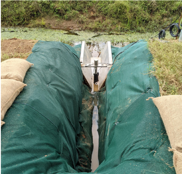
Figure 36. TriOS NICO installed in an RBC-200 flume, measuring nitrate concentrations and flow rates of water from an ag-pipe installed 1m below the surface.
