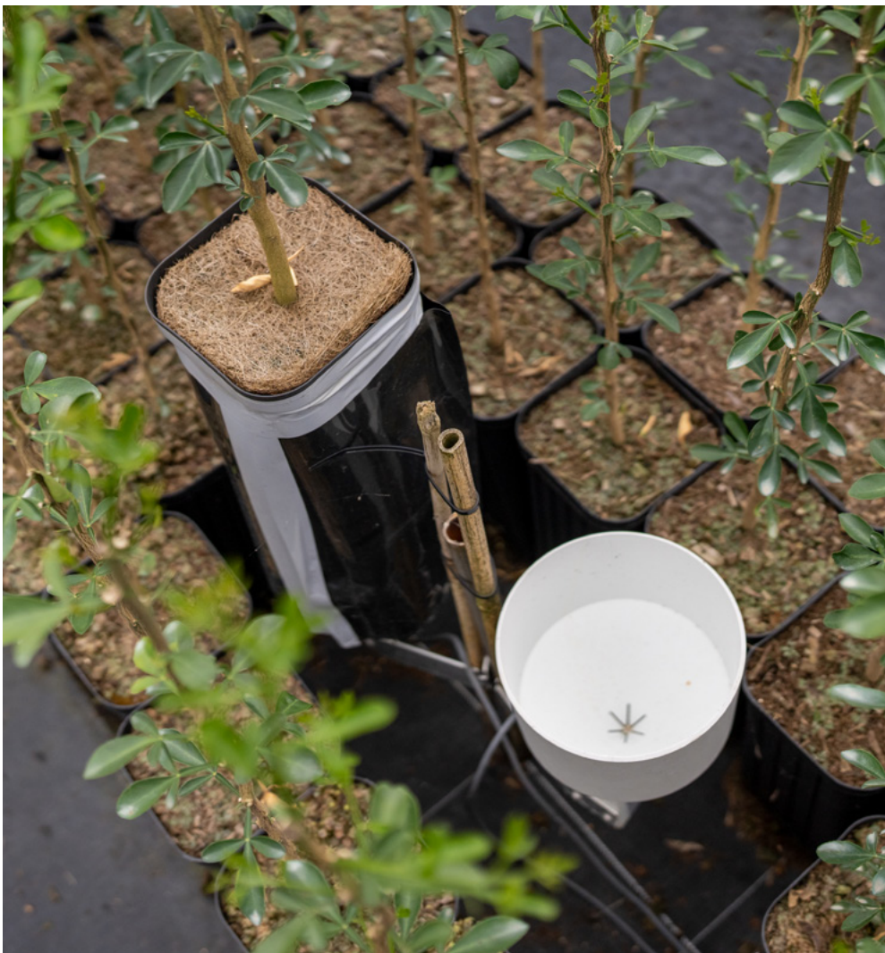
Figure 22. Two tipping bucket rain gauges used to measure irrigation volume applied to a container (left) and leachate volume from a container (right). Both tipping buckets are normally covered by a container and plastic shroud. Production nurseries often target a leachate fraction of 12%.
