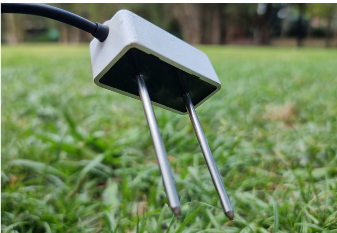
Figure 5. An example of portable, self-contained TDR soil moisture sensor.
