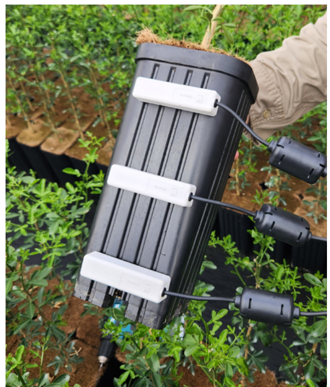
Figure 7. TDR moisture probes inserted into a plastic container.
