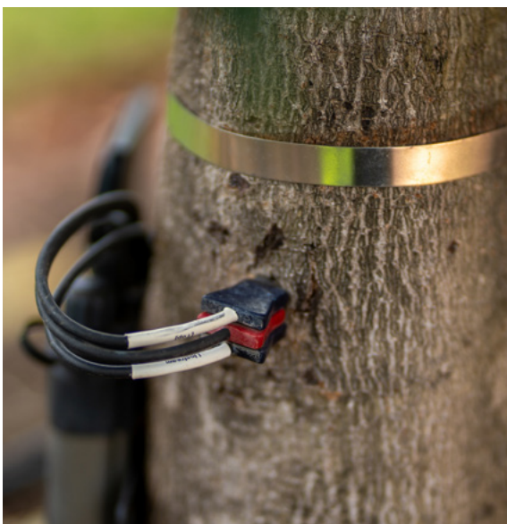
Figure 14. Sap flow sensor installed on an avocado tree, note the three prongs inserted into the trunk.
