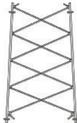
RST 20' Tapered Section Solid Round Legs & Angle Braces
