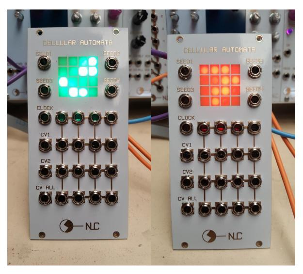
Left - 3mm narrow beam green LEDs Right - 5mm diffused red LEDs
