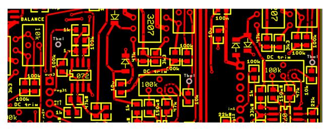
10. If you don't have an oscilloscope, patch in a clean sinewave and adjust BALANCE trimpot while listening to the output. Wherever it seems the least noisy will have to do.
