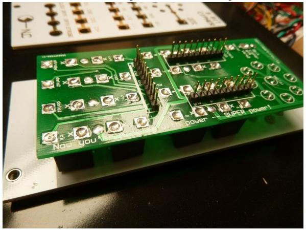
Remove the upper PCB and install the sockets & LEDs. It might be nice to install a different coloured LED for the centre (serial) position. I found it easiest to place the sockets on the PCB (unsoldered) then place the panel over them. It takes a little bit of jiggling, then hold the two together with one hand and screw the nuts on. Finally solder it all up.
