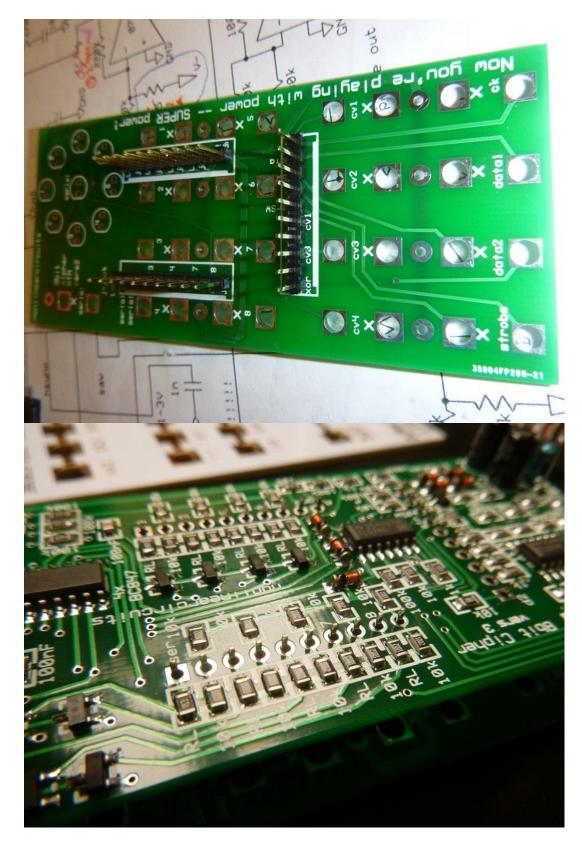
Place the other connectors onto the engine PCB, do not solder them yet
