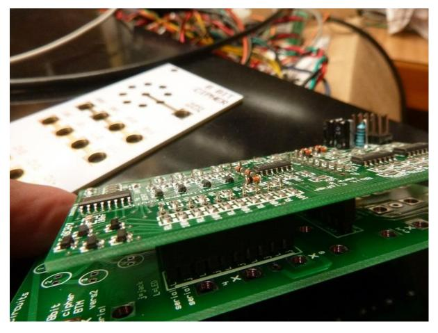
Connect the PCBs and when nice and snug, solder the connectors to the engine PCB
