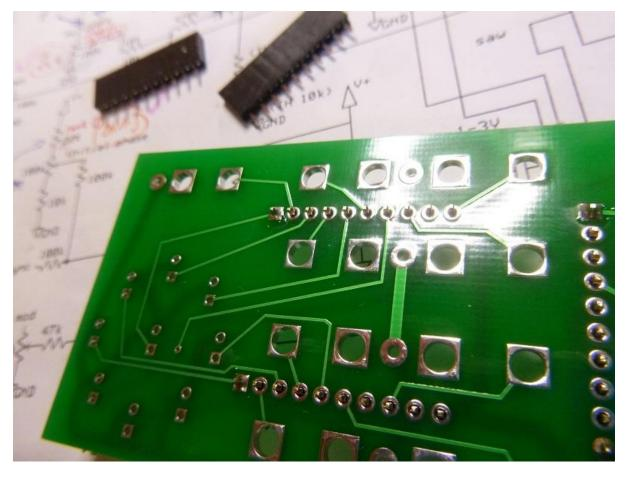
Place the connectors on the bottom PCB, solder the 2 end pins 1st and check they are standing perpendicular to the PCB. Correct if necessary and then solder the rest.
