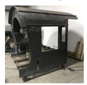
at their shop in Chattanooga earlier this year. The original cab was too far deteriorated to restore without losing most of the original materials so by building a new cab the original can be preserved and eventually be put on display. FMW Solutions completed fabrication of the new locomotive cab at their shop in Chattanooga earlier this year.
