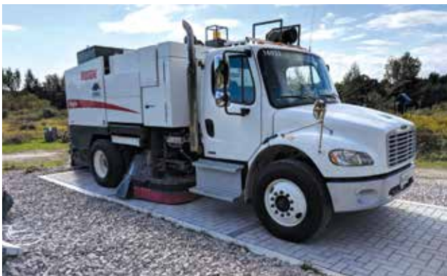
Figure 20. This type of mechanical sweeper removes sediment from joints parallel to the direction of the broom rotation.
