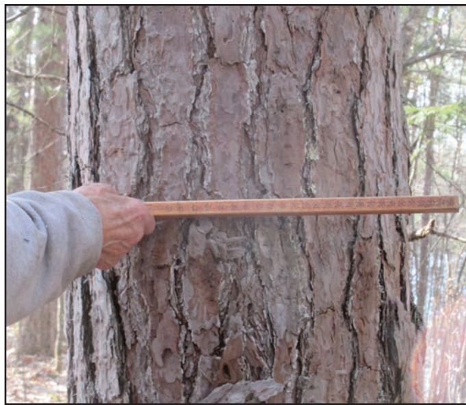
Red Pine saw timber, cruise stick displays 26" DBH (direction of eye). At 3 1/2 16' foot logs this tree could yield about 800 BF.
