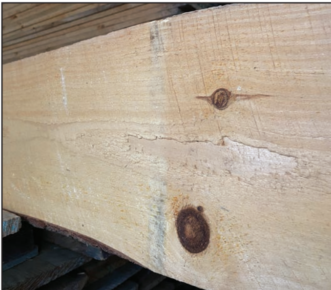
This rough-cut timber displays the marks of a sawmill blade.
