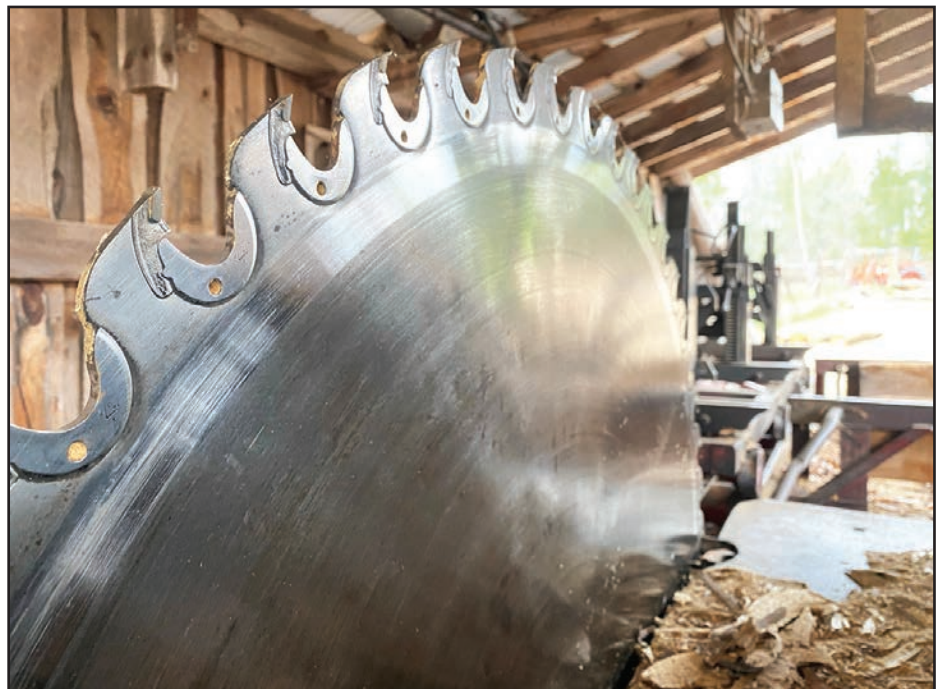
This functional sawmill has a 52" circle saw in style F and has 50 teeth made of carbide cutting tips which are held in place with individual shanks. This mill saws primarily Pine and uses a 120 horse power air cooled diesel power unit.
