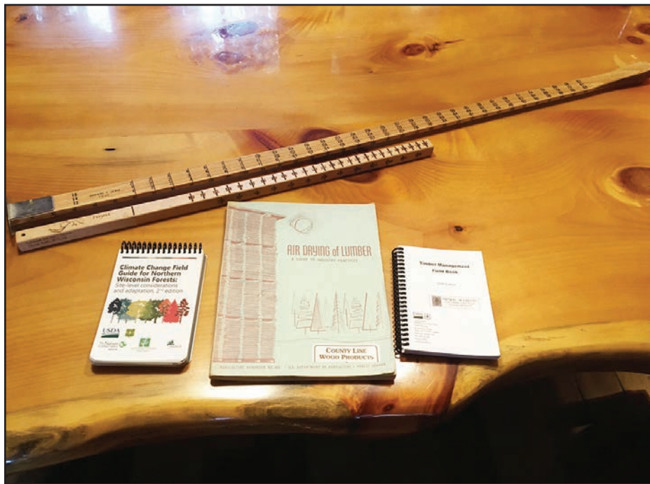
Scribner rule, handmade cruise stick, and manuals all assist in achieving sustainability in the process of log to finish product, and are displayed on top of a heavy White Pine table.
