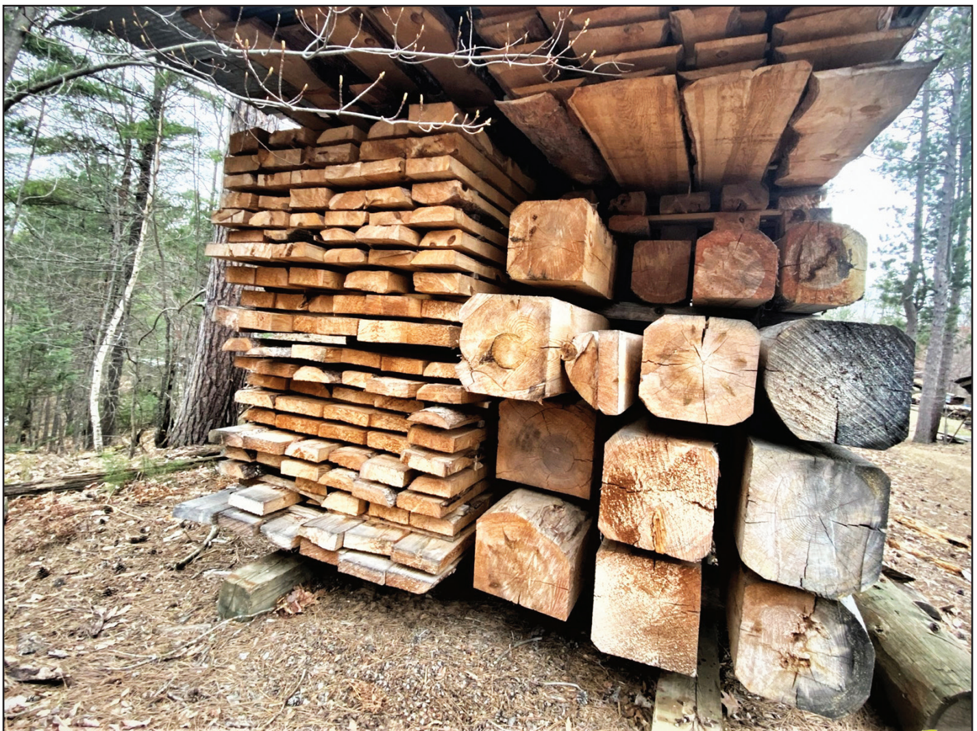
This pile of mix sized members includes potential re-saw beams on lower right. By re-sawing an oversize beam, the oxidation, stains, molds and dust are cleaned off and any warpage is also addressed.
