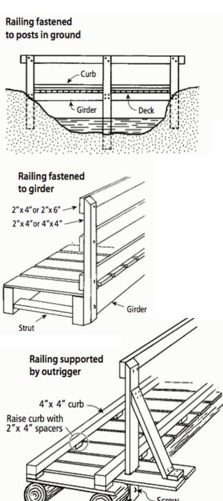
Figure 14-26. Curbs and railings make bridge crossings safer.
