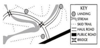
Figure 9-1. Example of a plan for a system of haul roads, skid trails, and log landings.
