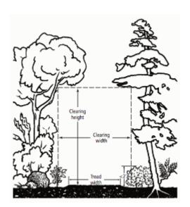
Figure 14-3. Tread width, clearing width, and clearing height.
