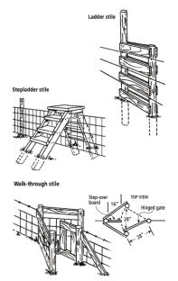
Figure 14-27 Hikers can easily use stiles to cross a fence.
