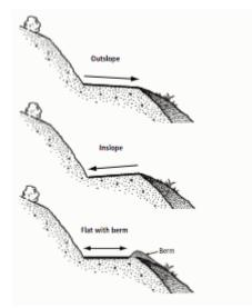
Figure 14-8. Outslope, inslope, and berm.
