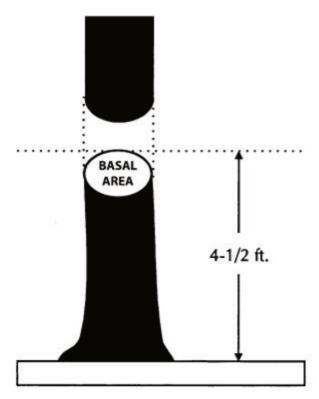
Figure 2-6. The basal area of a tree is its cross-sectional area measured 4.5 feet above the ground.
