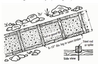
Figure 14-12. A climbing causeway allows you to hold fill material on a steep grade.
