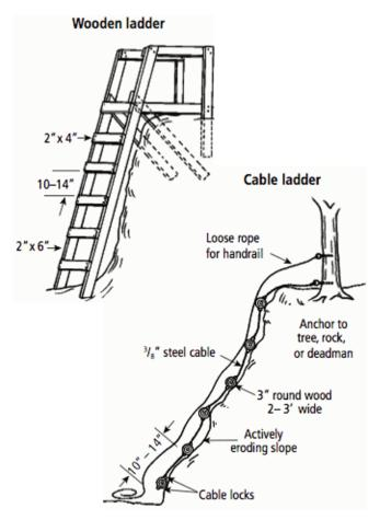
Figure 14-14. A ladder can be a good way to help hikers climb a steep slope.
