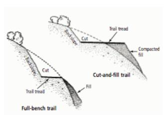
Figure 14-6. Full bench and cut-and-fill trails provide safe travel across steep slopes.
