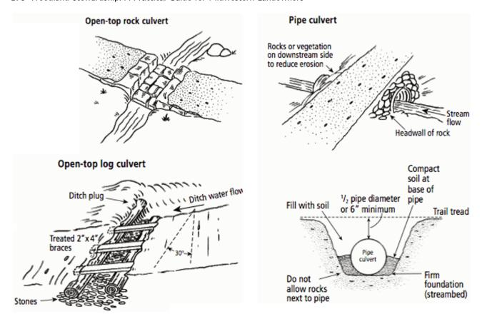
Figure 14-21. A culvert is a good option for crossing a narrow stream.
