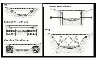
Figure 14-22. The best type of abutments for your bridge depends on the size of the bridge and the surrounding conditions.
