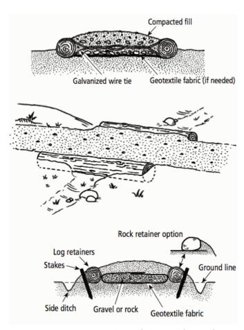
Figure 14-17. A causeway (turnpike) raises the tread above wet soil.
