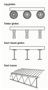
Figure 14-23. Girders and trusses support the bridge deck.
