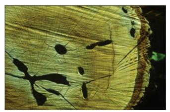
Figure 7-8. Wood-boring insects destroyed most of this oak log's value. photo: Don Breneman.
