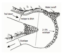
Figure 14-11. Switchbacks help the user climb a steep slope at a comfortable grade.
