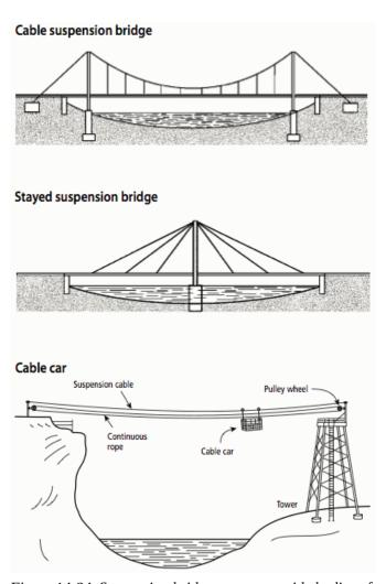
Figure 14-24. Suspension bridges can span wide bodies of water.
