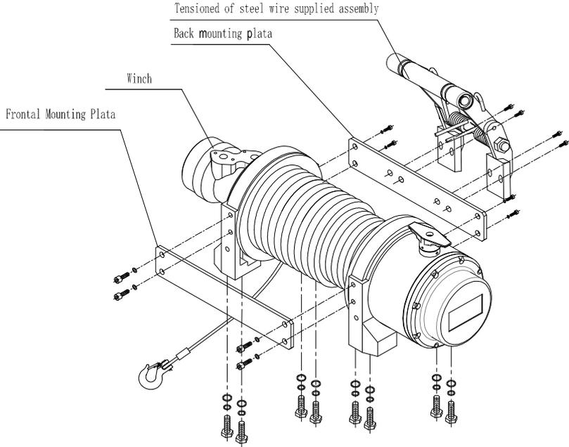
**Below is installation illustration with roller fairlead of 10000NW:**
