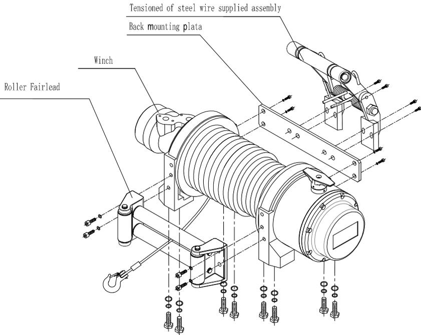
**Below is installation illustration of 15000NW:**
