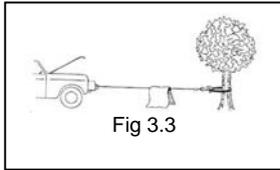
When pulling a heavy load, place a blanket or jacket over the wire rope five or six feet from the hook. In the event of a broken cable it will dampen the snap back. For additional protection open the hood of the vehicle as shown in Fig 3.3
