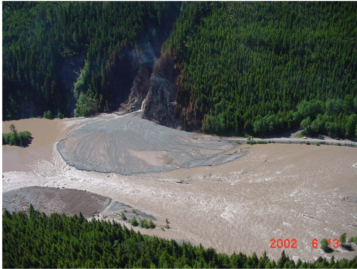
Figure 5. A 2002 rock slide – debris flow ruptured a natural gas pipeline and resource road adjacent to Zymoetz River. Note the debris fan in the river. Photo: Marten Geertsema
