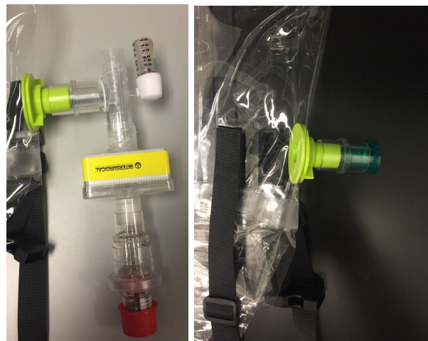
Figure 2.4: (left) Connection of the manometer, HEPA filter, and PEEP valve in series at the expiratory port for wall oxygen interface (right) plugged expiratory port for ventilator interface.
