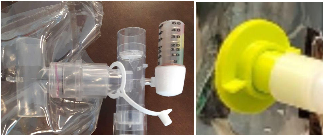
Figure 2.2: (left) T-piece connector and 22mm ID port (right) 3D printed port
