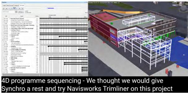
Using this 4D approach enabled debate and discussion with suppliers to ensure construction sequencing could be optimized between work packages, logistics and safe working zones could be tailored effectively and safely, responsibilities could be verified, along with providing an overview of how the IoT would be built day by day, which meant everyone was better informed and had a common understanding from which they could meaningfully contribute.
