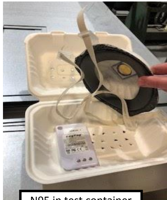
N95 in test container with data logger
