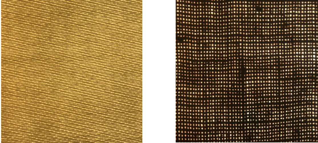
Image 1: Light visibility through a more dense fabric (left; 200 threads per inch (tpi) cotton pillow case), and less-dense fabric (right; 60 tpi open-weave cotton)
