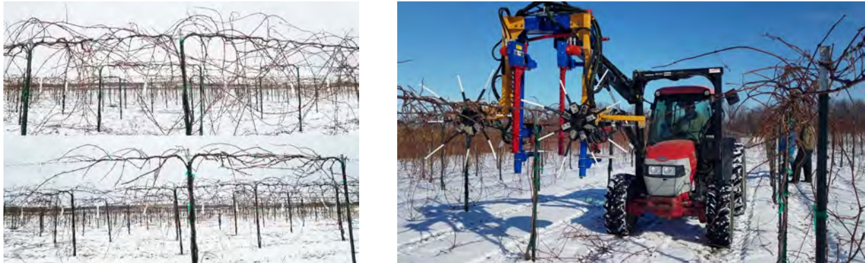
Figure 1: Dormant Concord grapevines before and after mechanical pre-pruning (left top and bottom) with an OXBO V-Mech sprawl pre-pruner (right).
