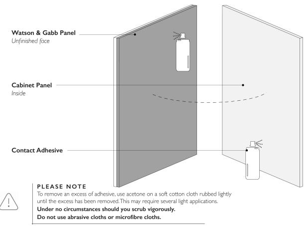
When the panel is fixed in position, **veneer rollers** should be used to ensure adhesion between the two surfaces. Work from the centre of the panel outwards to the edges for maximum strength of bond.
