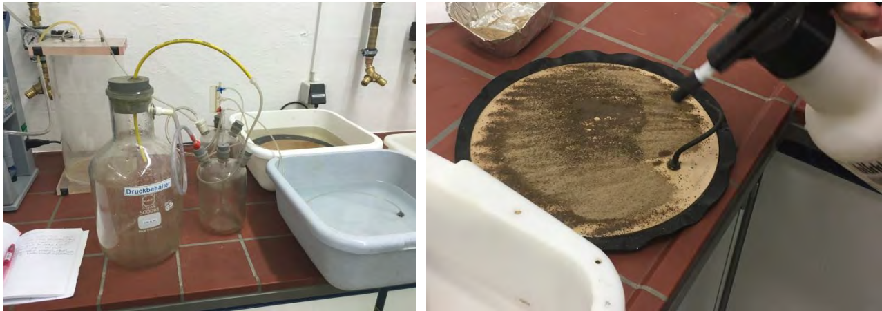
Figure 34: Conditioning of pressure plates prior to experiment with negative pressure (left) and preparation of ceramic plate with kaolin salt-mixture and water (right)
