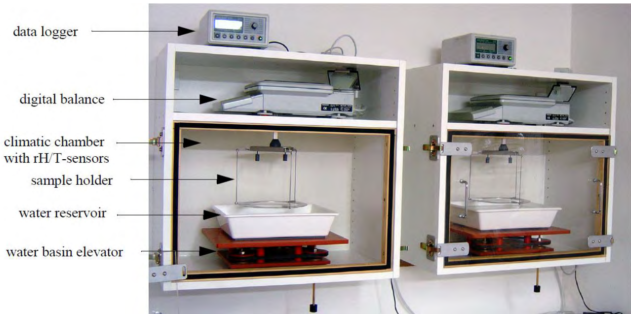
Figure 32. System for automatic measurements of water uptake coefficient (Rudolf Plagge, Scheffler, & Grunewald, 2005).
