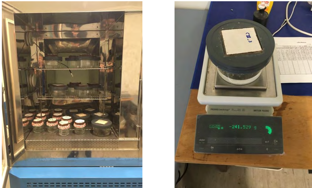
Figure 31. Cups with specimens in climate chamber (left), and cup being weighed (right).
