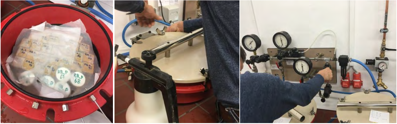
Figure 35: Specimens in pressure plate apparatus, covered by wetted towels (left), the lid of the pressure plate apparatus being sealed tightly (middle), and pressure being applied to the system (right)
