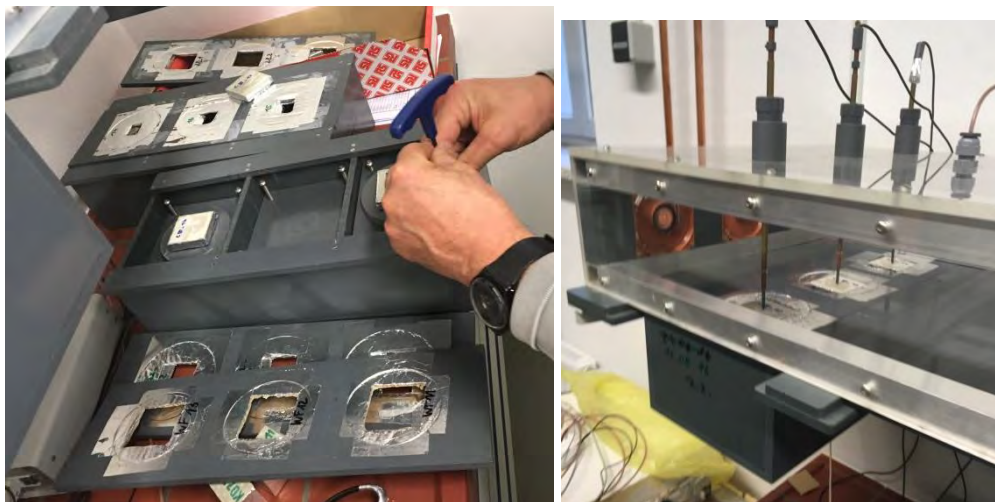
Figure 44: Adjustment of the drawer for the specimens (left), and drawer with specimens placed in climate chamber, and surface temperature sensors in place.
