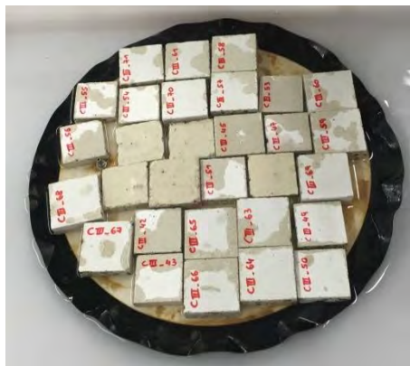
Figure 37: Saturation of specimens on ½ bar ceramic plate, partially immersed in water
