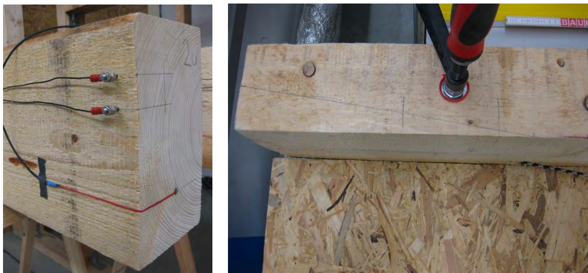
Fig. 10.: Mass-related wood moisture content measurement in the front end of the beam (left) and preparation of the combined sensors behind the front face of the beam (right).
