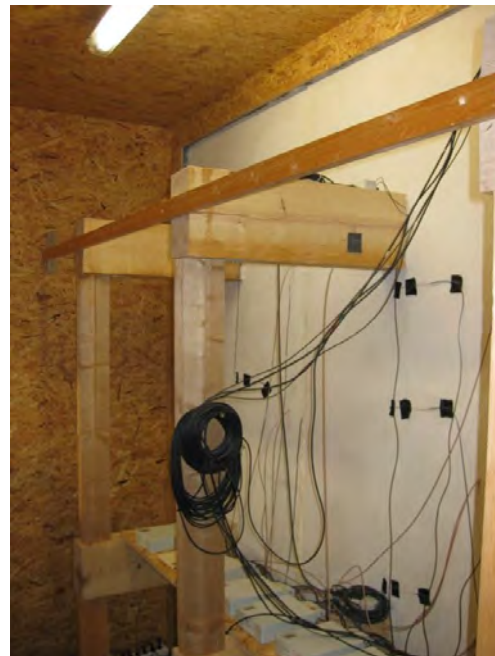
Fig. 4.: Cold-side chamber (left) with de-humidifier (dark grey device), air inlet (behind vents) and heating unit (white device). Warm-side chamber showing wires of the measurement equipment in the wall and with the beam ends supported by a wooden auxiliary construction.
