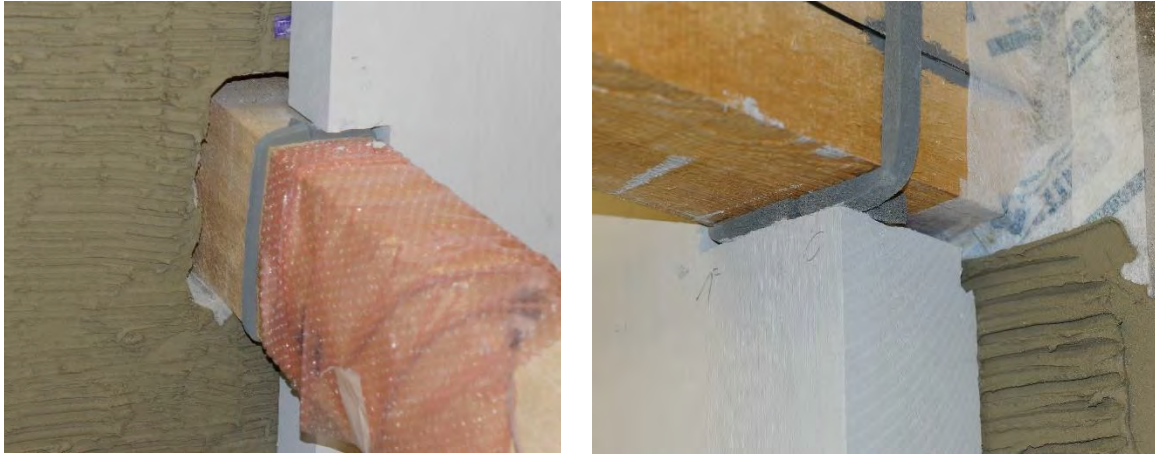
Fig. 11.: Sealing variants in test strip 2 (Calsitherm) for the lower joist end (left) and for the upper joist end (right).
