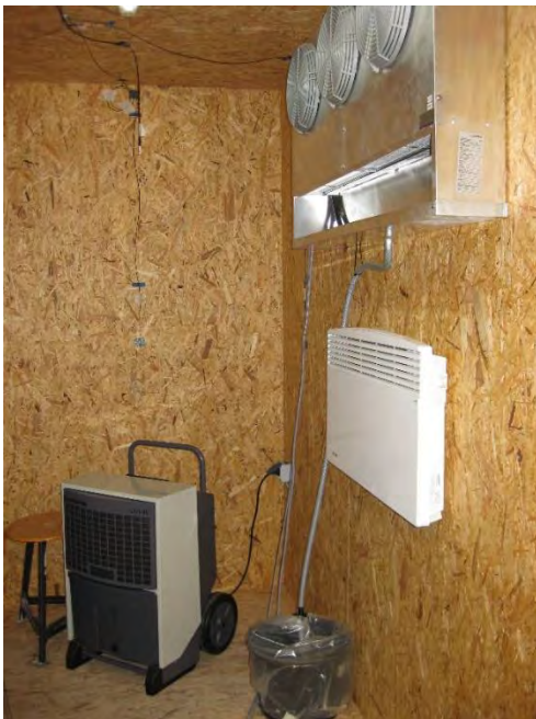
Fig. 4.: Cold-side chamber (left) with de-humidifier (dark grey device), air inlet (behind vents) and heating unit (white device). Warm-side chamber showing wires of the measurement equipment in the wall and with the beam ends supported by a wooden auxiliary construction.
