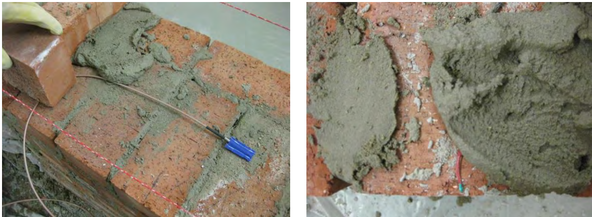
Fig. 5.: Combined temperature and relative humidity sensors in the masonry: sensor with protective casing in the middle of the masonry (left) and near-surface sensor (right)
