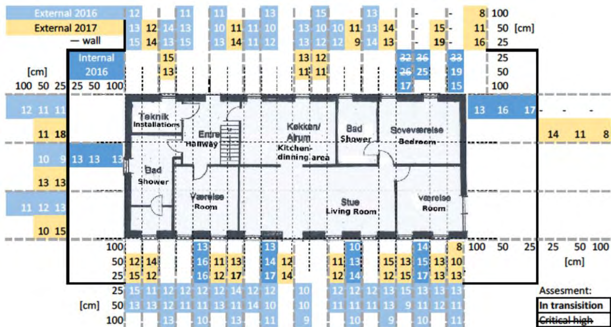
Figure 56: Troxler measurements before insulating and again after insulating. The first values in a double column (shown with faded and thick dashed line) contain 2016 and 2017 measurements (e.g. upper left: 12, 13, 15 & 12, 14) measured in the middle of the covered wall length while the following single column include 2016 and 2017 measurements (e.g. upper left: 14, 13 & 15, 13) below the window. The third column only include measurements from 2016. Heights stated are measured from the foundation. Yellow boxes are placed where possible due to space limitations. Values from 17 to 25 are assessed as in transition between non-critical and critical moisture content for bricks while above 25 is critical.
