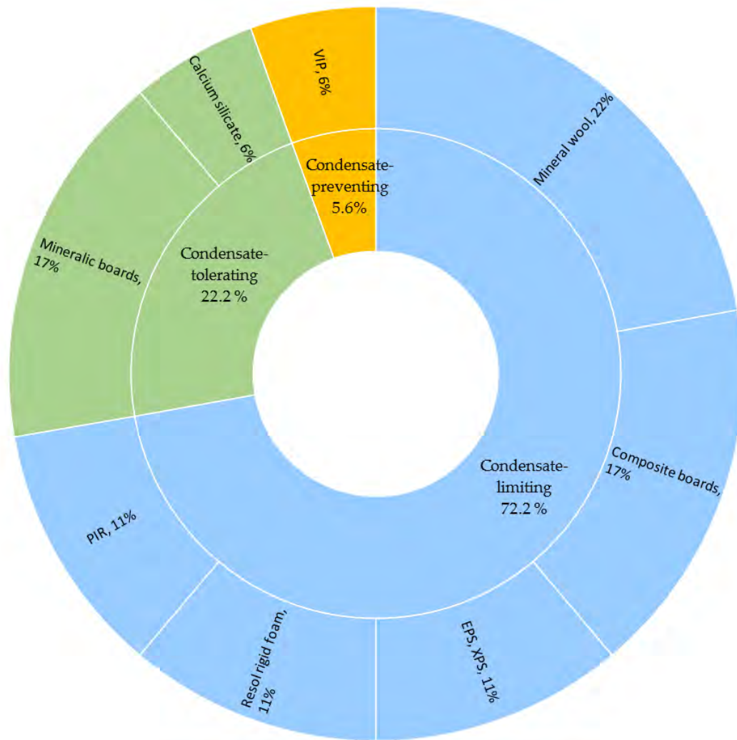
Figure 20: Sunburst diagram showing the share of different insulation systems in RIBuild case studies grouped by their insulation system class: condensate-tolerating (green), condensate-limiting (blue) and condensate-preventing (orange).
