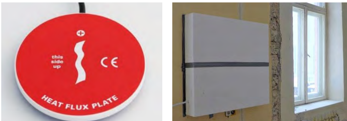
Figure 48: Heat flux sensor and heated box setup used on the west facade of the RIBuild case study building Catholic Seminar in Riga.
