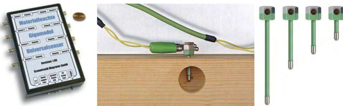
Figure 52: 8-fold extension module, measuring cables and electrodes to measure moisture content in masonry and rendering.
