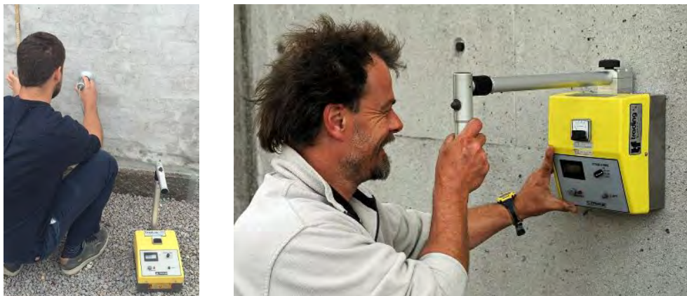
Figure 57: Troxler measurement tool standby while other measurements are carried out (left). Troxler equipment in use (right) (Brandt & et al., 2013).
