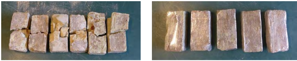
Figure 62: Bricks after 15 frost-thaw test cycles. Left: Fully saturated samples (~36%). Right: Samples saturated to 20%.
