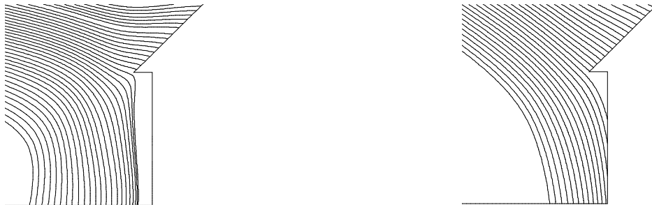
Figure 4–25: Visualisation of rain trajectories on a façade in case of a roof overhang. For small droplets in a low velocity wind field (left figure) the roof overhang shields the façade completely for impinging rain droplets. For larger droplets in a high velocity wind field (figure at the right) shielding is less, but still larger than the geometrical shielding.
