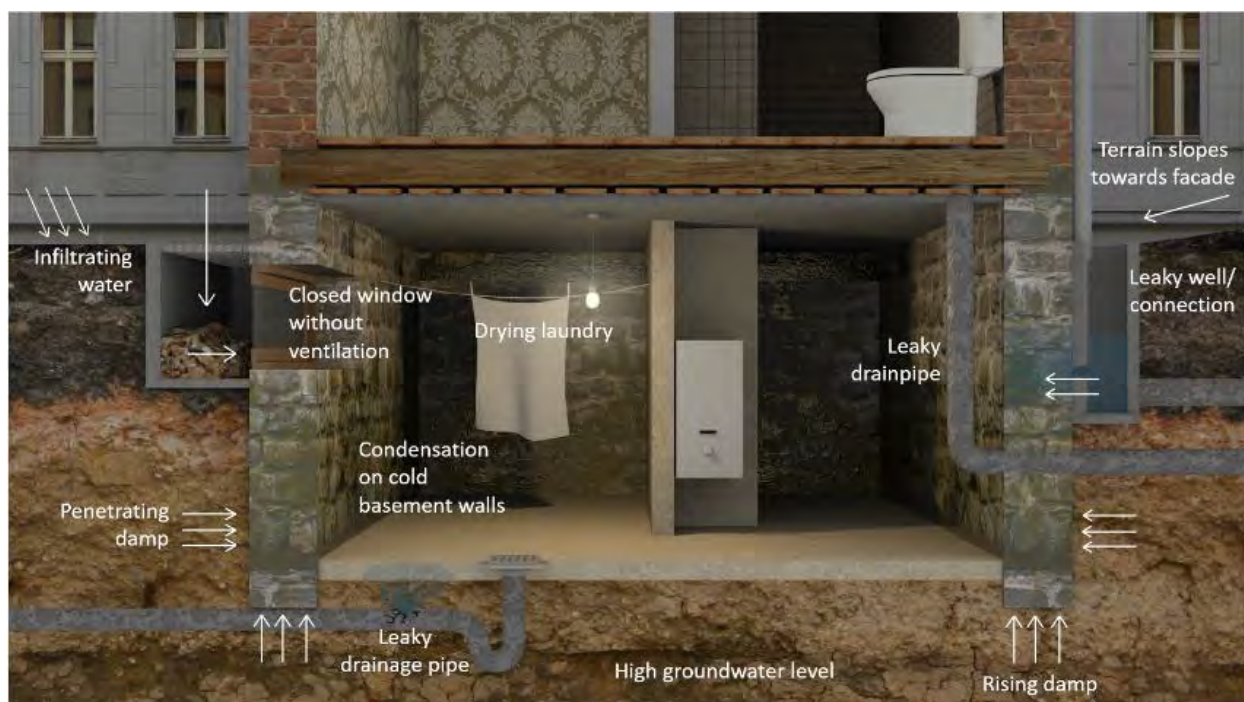
Figure 4–20: Possible moisture sources in basements ( https://gi.dk/Publikationer/Standning%20af%20Grundfugt_web.pdf )
