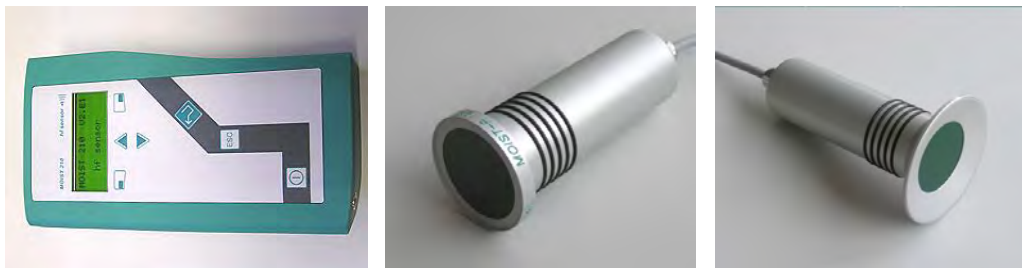
Figure 4–45: Example of a microwave moisture analyser with different measuring heads (Source: hf-sensor.de)
