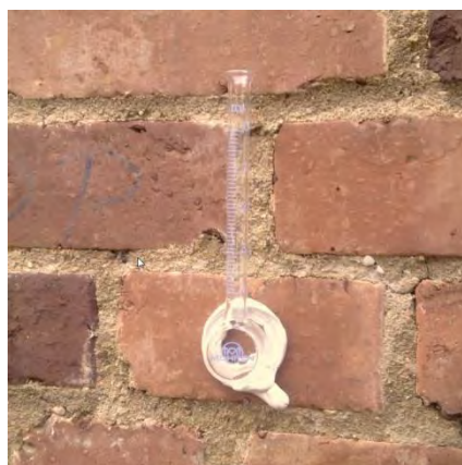
Figure 4–46: Test tube according to Dr. Karsten, placed on a brick
