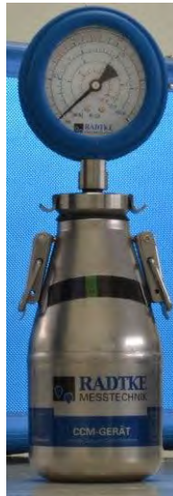
Figure 4–49: Example of a CM measuring instrument for moisture measurement (Source:radtke-messtechnik.com)
