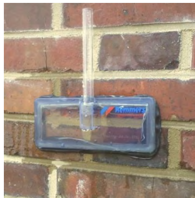
Figure 4–47: Test plate according to Franke, detection of brick and joint content
