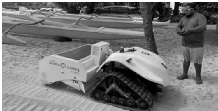
A remote-controlled, 100% electric robot that runs on solar and battery power, the BeBot emits zero emissions and does not cause beach erosion due to its track system.
