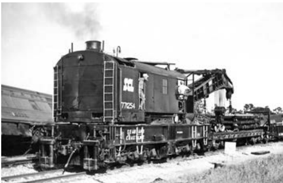
Above: Steam-powered crane SCL 765150 and its boom flatcar, ACL 65220, were among the wrecking equipment brought in to quickly clear the mainline. The 150-ton-capacity 765150 was assigned to Lakeland, Florida, and was formerly ACL 65229, a 1919 product from Bucyrus-Erie. —Joseph L. Oates photo
