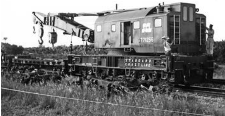
Right: SCL 771256, a year-old diesel-powered crane that was ex-SAL 71982, was one of two such 250-ton cranes Seaboard purchased just before the merger from American Hoist & Derrick. No. 771256 was assigned to Wildwood, Florida. — Stan Jackowski photo
