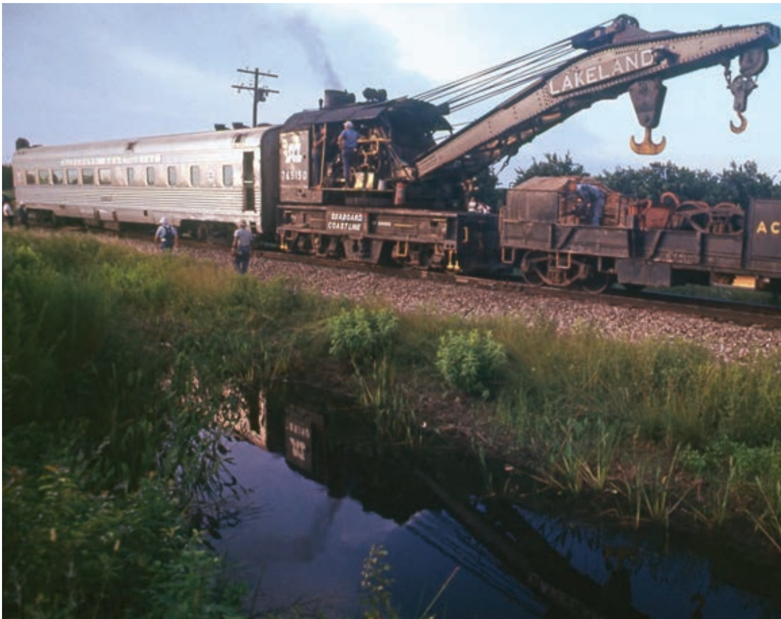
Above: Steam-powered crane SCL 765150 and its boom flatcar, ACL 65220, were among the wrecking equipment brought in to quickly clear the mainline. The 150-ton-capacity 765150 was assigned to Lakeland, Florida, and was formerly ACL 65229, a 1919 product from Bucyrus-Erie. —Joseph L. Oates photo
