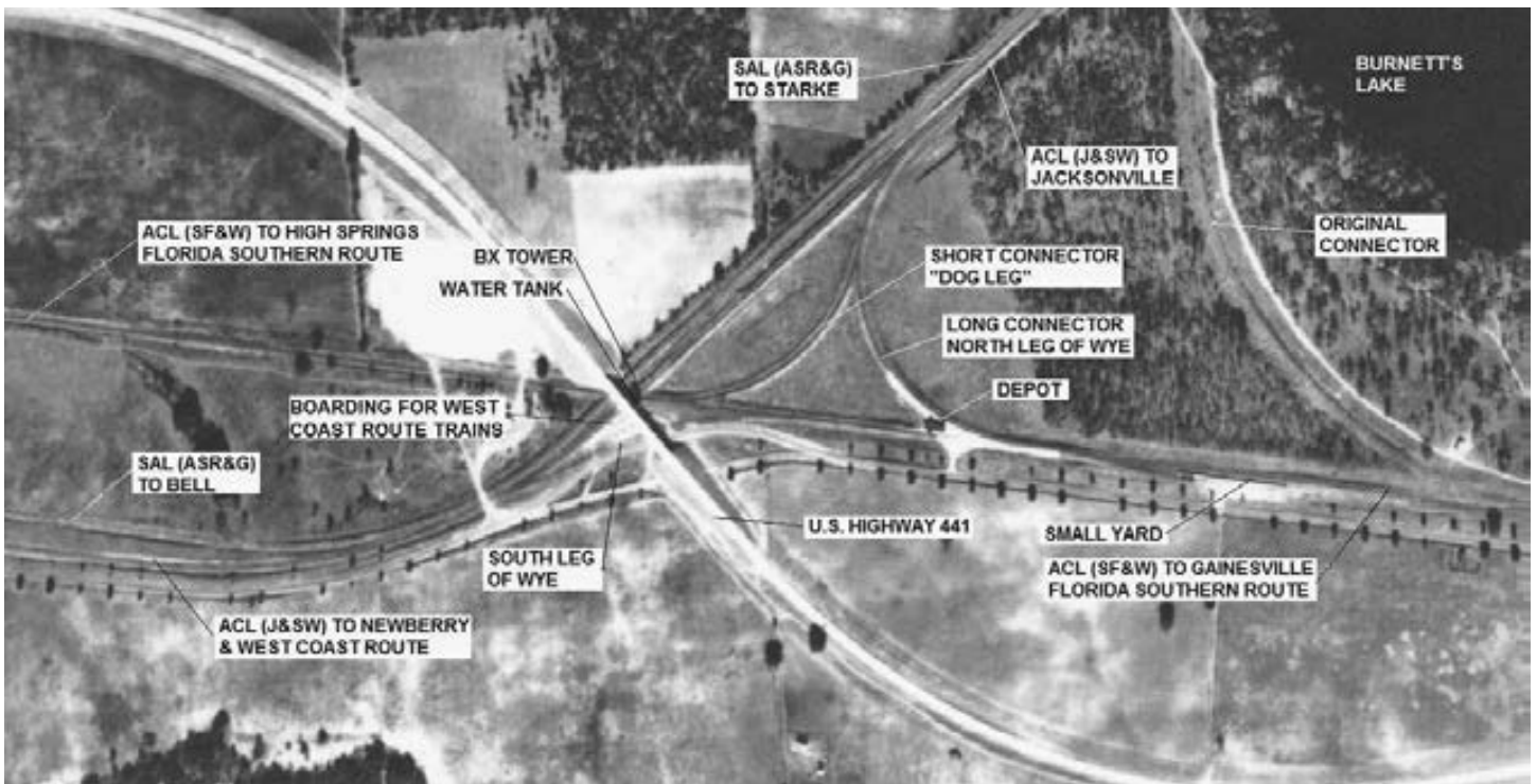
Above: This 1937 aerial photograph, with north at the top, clearly shows the track layout of Burnett's Lake Junction and the U.S. 441 overpass crossing over diamonds and the south leg of the wye. The water tank and tower are in the shadow of the overpass. Burnett's Lake is in the upper right. The abandoned remains of an earlier connecting track can be seen closer to Burnett's Lake and are thought to be the original connection. The town of Alachua is about a mile to the left of the junction. Although the ACL (SF&W) route runs nearly east-west at Burnett's Lake, the line to High Springs (at left) soon turns toward the northwest, and the line to Gainesville soon curves to the southeast. — University of Florida aerial photography collection
