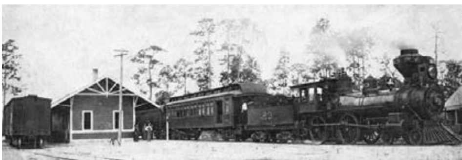
This Jacksonville & Southwestern train is at the J&SW Newberry depot circa 1900. The locomotive is 4-4-0 No. 23, an 1887 Baldwin product, purchased used from the Wichita & Western as that road's No. 7. One of eight locomotives owned by the J&SW, No. 23 became ACL class D-7 543, and was later sold to the Aberdeen & Rockfish. The train had made its 87-mile run from Jacksonville through Burnett's Lake to Newberry and had been turned, and was ready to make its return run. —Florida Archives photo rc12968
