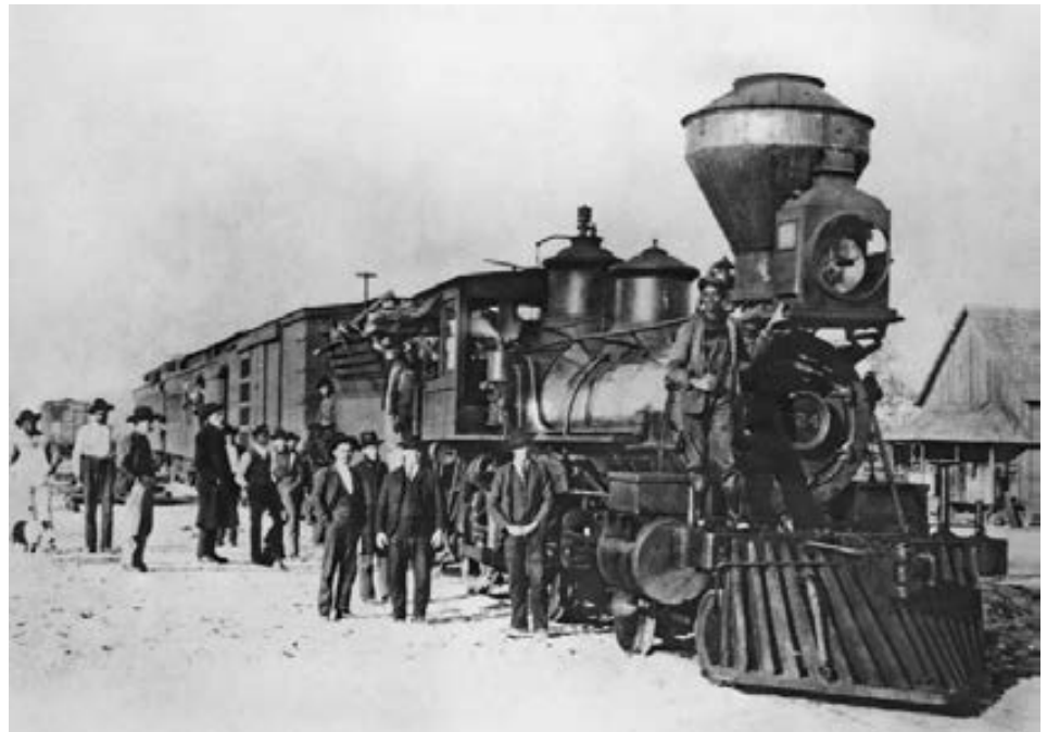
The Atlantic, Suwannee River & Gulf's mixed train was at Starke with Florida Central & Peninsular Railway's 4-4-0 324 on the head end, ready to depart on its 55-mile trip to Wannee in 1905. The 324 was built by Rogers in 1885 for the Florida Railway & Navigation Company, a predecessor of the FC&P. The FC&P was under control of the Seaboard Air Line at this time by stock ownership. — Ken Murdock collection
