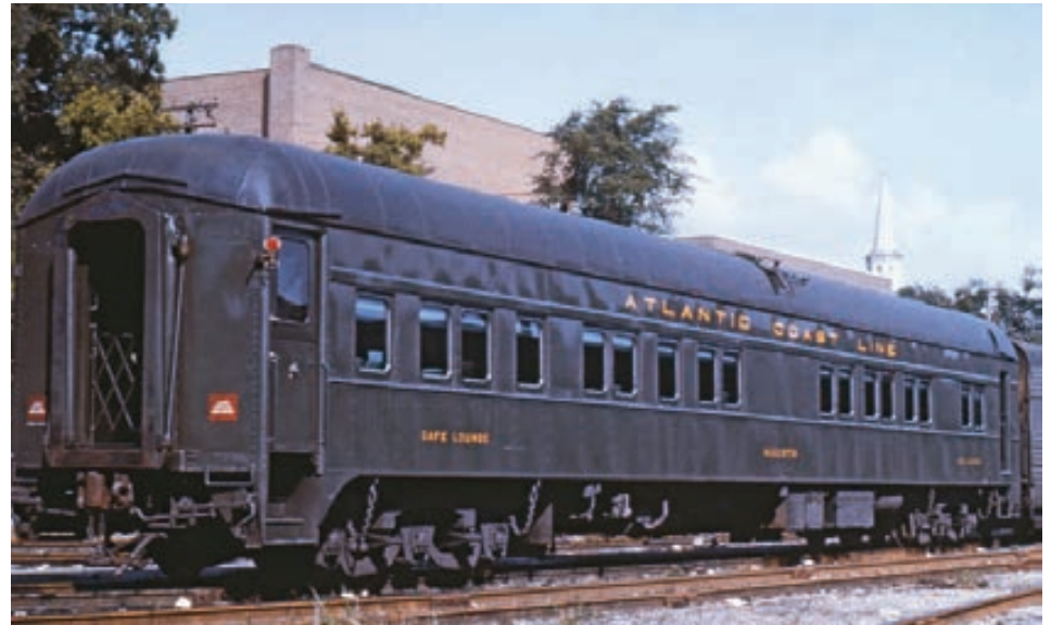
Above: Café-lounge Augusta was one of two similar cars that ACL rostered to serve light meals on secondary trains, making the cars well suited for the Florence–Augusta run and other assignments on other secondary trains in the Carolinas. The car had 24 dining seats and 20 lounge seats, and is seen here in its namesake city about 1966. —R.H. Hanson collection
