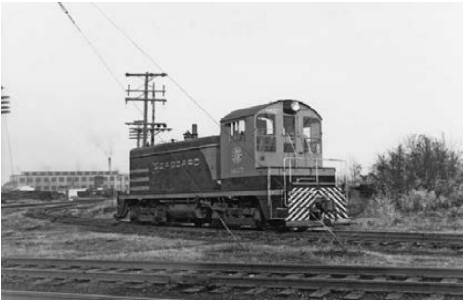
Left: Seaboard NW2 1407, a 1942 product from EMD, is switching at the large Portsmouth yard and shop complex. The huge back shop building is in the left background; it was considered a state-of-the-art steam locomotive repair facility when built in 1916. —Robert Wayne Johnson photo
