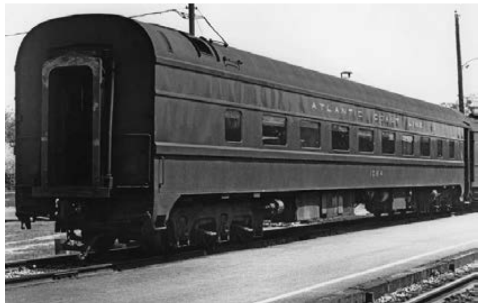
Below: No. 1084 was one of 25 class A-15 heavyweight coaches ACL extensively rebuilt in the early 1950s from cars originally delivered in the 1920s. They had interiors equivalent to Coast Line's lightweight cars and were common sights on secondary runs. The car was photographed at Augusta during April 1969. —A.M. Langley Jr. photo
