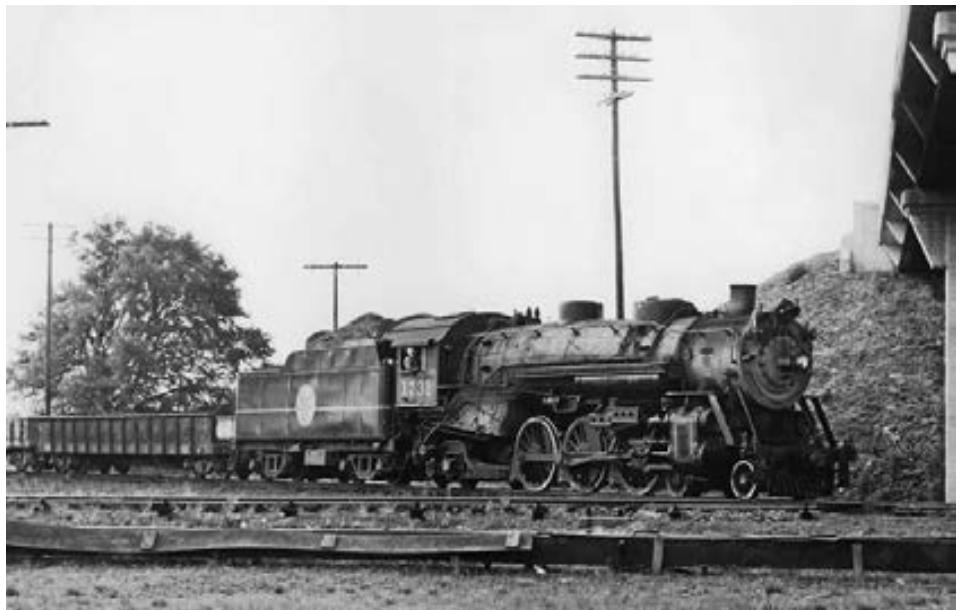
Below: This southbound freight, powered by ACL P-5-B 1731, departed High Springs and is about to pass under the U.S. 441 bridge as it enters Burnett’s Lake junction in 1949. The SAL track to Bell is seen crossing immediately in front of the locomotive. ACL’s J&SW line, which parallels the SAL, is mostly hidden by the wooden structure in the foreground that runs parallel to the track. — Russell Tedder collection
