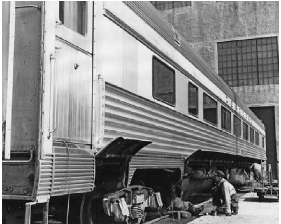
The Portsmouth shops were a major SAL repair facility, and in later years were the primary passenger car shops for the system. This circa-1950 scene shows a lightweight coach in the shops for repairs; note the temporary shop trucks being used and the car's skirting raised for access to the underbody. —SAL photo, Robert Wayne Johnson collection
