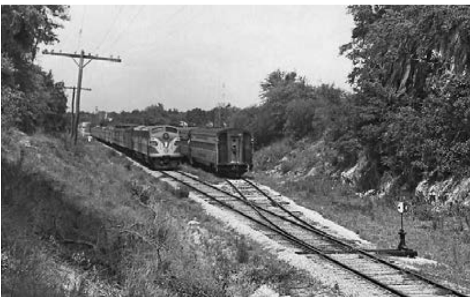
Left: The St. Petersburg sections of ACL's West Coast Champions are meeting and passing on the West Coast Route in dark territory on this siding with hand-thrown switches just south of Leesburg. Meets didn't usually occur at this location but northbound No. 192, on the right, is running about an hour late as it passes southbound No. 191 on the left, circa 1957. Train 192 will pass through Burnett's Lake in about two and a half hours as it makes its way to Jacksonville to join the main (Tampa) section of the WCC . The last car on No. 192 is one of ACL's Beach -series 6 double bedroom-bar-lounges distinguished by their unusual triple-porthole end doors. —John Rapalje photo, Central Florida Railway Historical Society collection
