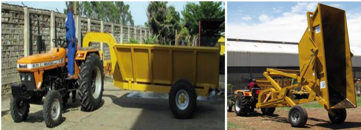
**Plate 6: Sample of tractor and trailer system for Malindi:** Tractor drawn low loading height trailer for door to door manual loading or pay as you through and high tipping trailer skip picker.
