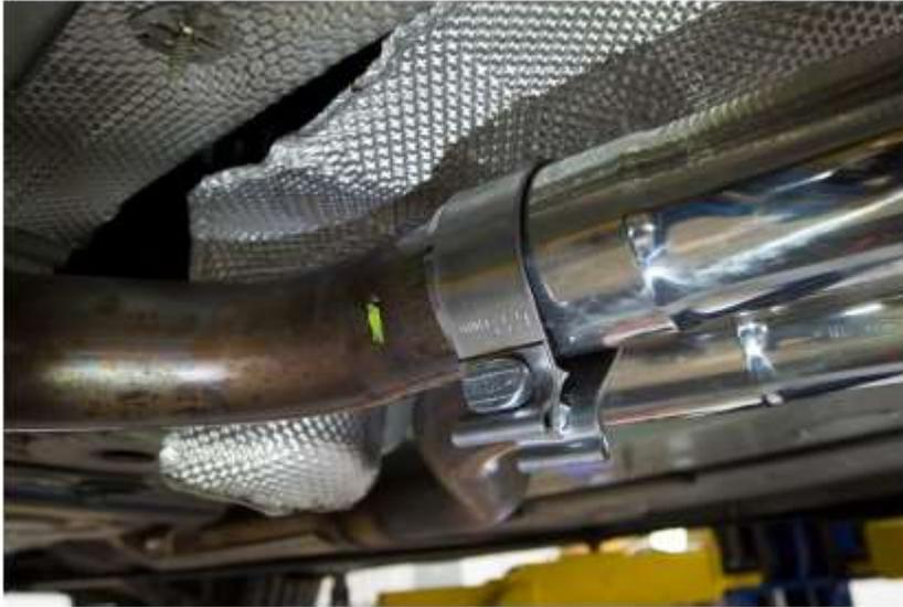
8. Align and slip URUTU X-Pipe onto rear factory tubing.
