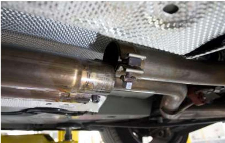
6. Separate the front joint of the resonator section and remove the factory resonator.
