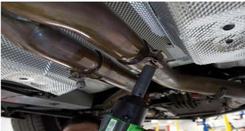
4. Loosen front exhaust joint clamps in front of the factory resonator.
