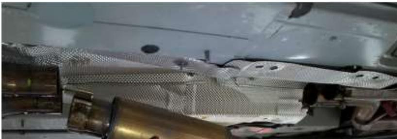
7. Slip URUTU X-Pipe over the front factory tubing.
