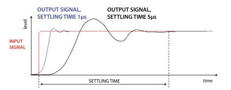
Figure B: Pulse response of an audio signal after transfer through various analog and digital systems.
