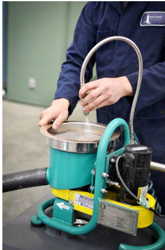
Figure 4.1 - Knelson MD-3 Concentrator at Blue Coast Research
