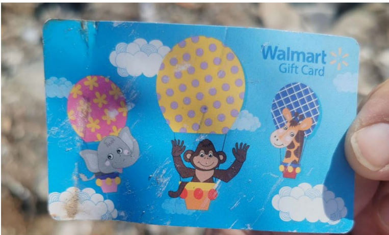
This Walmart gift card was found dumped in Turkey. Infrared testing confirmed that it's made of PVC. Turkey is one of the many countries that have banned imports of PVC plastic waste.
