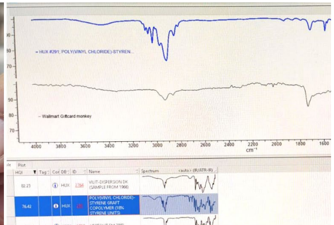
This Walmart gift card was found dumped in Turkey. Infrared testing confirmed that it's made of PVC. Turkey is one of the many countries that have banned imports of PVC plastic waste.
