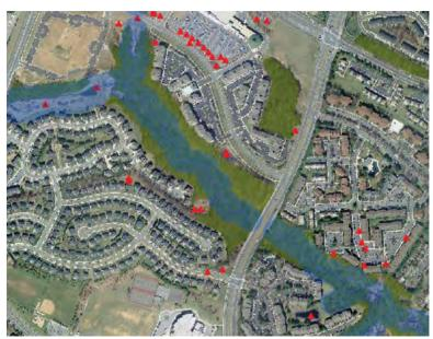
The red triangles represent stormwater BMPs; the green area represents the vegetated riparian buffer; and the shaded blue area indicates a buffer zone of 100 feet on either side of the stream as a reference. (HW graphic)
