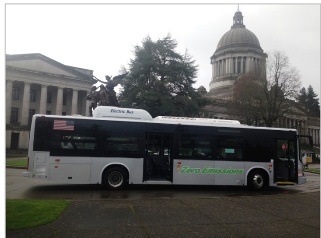
BYD Motors demonstrates its 40-foot electric bus with 150 miles of range and zero tailpipe emissions at the Electric Vehicle Showcase in Olympia, Washington, on February 25, 2014.
