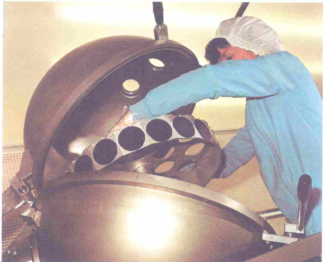
MOS integrated circuit production at Mullard, Southampton. Ion Implanter. Ions of boron, arsenic, etc, are implanted into the surface of the silicon wafer to form doped regions.
