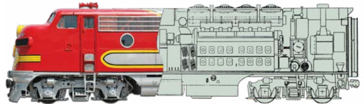
Partial cutaway view of the Museum's Santa Fe F-7A diesel-electric locomotive. Built by General Motors' Electro-Motive Division, 1952.
