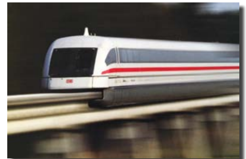
New technologies employ the use of magnetism to levitate and propel high speed trains. Known as Mag-Lev, this form of rail transportation can safely move passengers at speeds of up to 300mph through a linear induction process.
