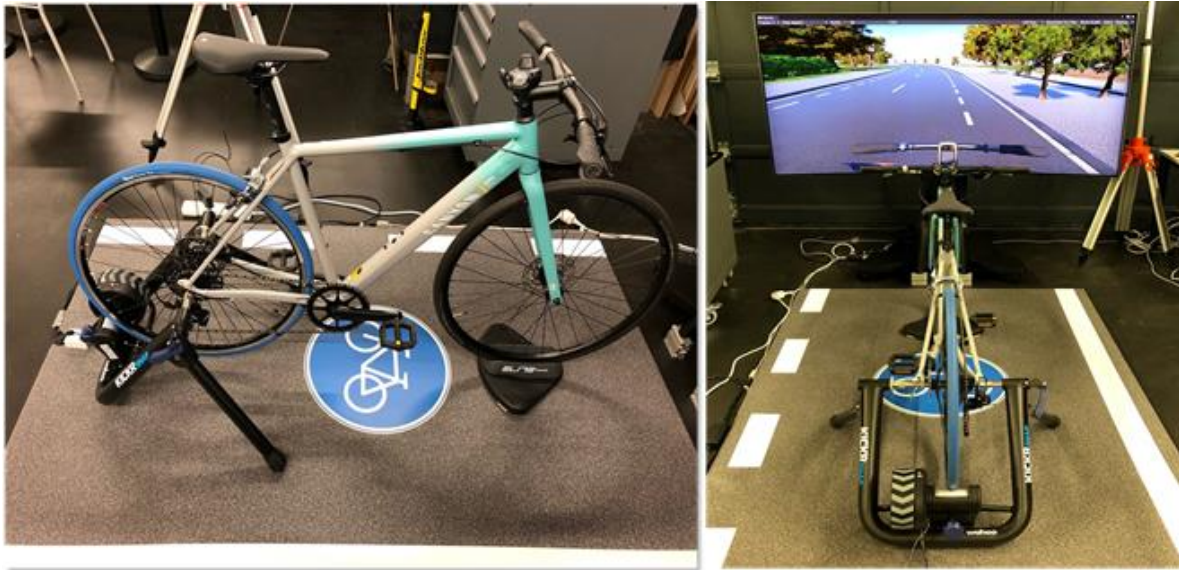
Figure 9. Virtual reality bicycle simulator
