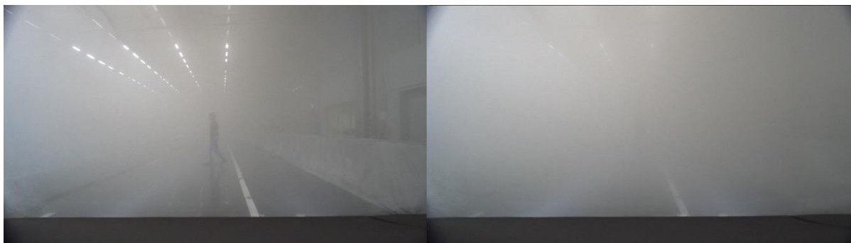
Figure 12: Exemplary camera images taken at low fog density (left) and high fog density (right).
