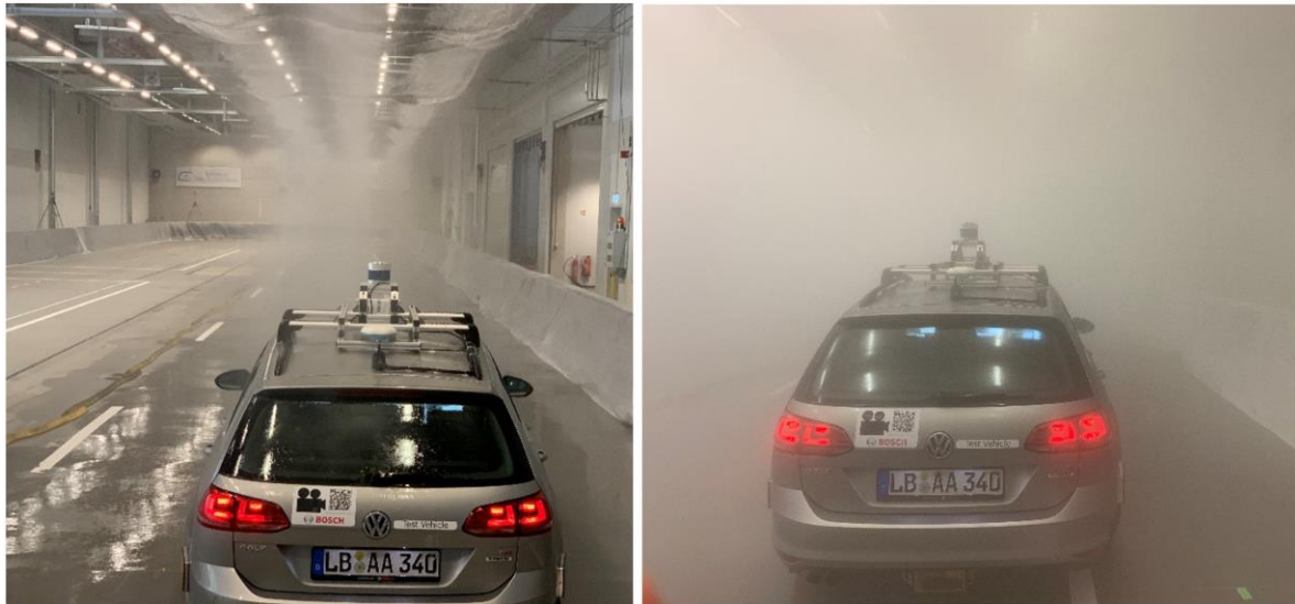
Figure 4: SAFE-UP tests under adverse weather conditions with a rain rate of 98 mm/h and a fog density with a resulting viewing distance of 5m.
