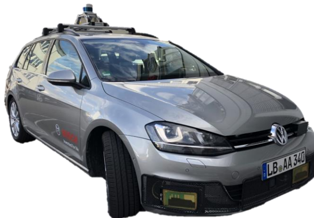
Figure 1: The Demo 2 vehicle : a Bosch development vehicle with prototype high resolution radar, stereo video setup and lidar sensor.
